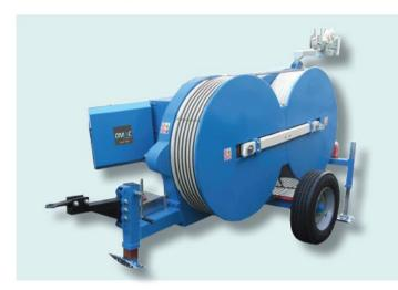
Hydraulic tensioner fit to string one conductor or fiber optic cable. One hydraulic circuit allows to tension at constant force even varying the speed of stringing.
