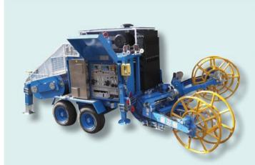
Hydraulic puller fit to pull one or two ropes in stringing operations of overhead transmission lines. Two hydraulic circuits allow to continuously vary the speed in both directions by operating two independent control devices. The two circuits may also be matched and operated together by one control device.
