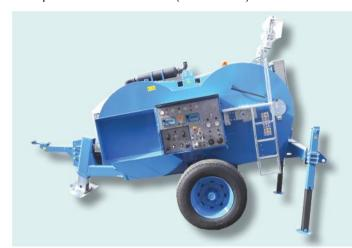
Hydraulic machine designed to operate both as a tensioner and as puller, fit to string one or two ropes or conductors.
