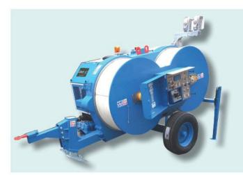
Hydraulic tensioner fit to string one or two conductors or optical fiber cables. One hydraulic circuit allows to tension at constant force even varying the speed of stringing. Equipped with engine for pull-back performances.
