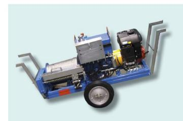
Hydraulic winch fit to pull one rope in service operations such as setting-ups and adjustment of transmission lines and underground cables laying. The winch can be disassembled into three parts. One closed hydraulic circuit allows to continuously vary the speed in both directions by operating one control device.
