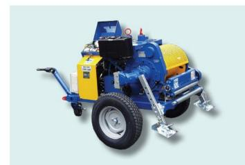
Hydraulic winch fit to pull one rope in service operations such as setting-ups and adjustment of transmission lines and underground cables laying. Direct pull on the drum. One closed hydraulic circuit allows to continuously vary the speed in both directions by operating one control device.
