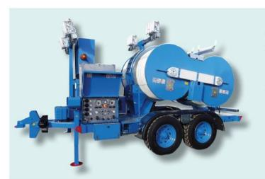
Hydraulic tensioner fit to string 1, 2, 3 or 4 (up to 6 on demand) conductors. Two hydraulic circuits allow to tension at constant force even varying the speed of stringing. The two circuits can be used independently or simultaneously, with with automatic forces partition. Equipped with engine for pull-back performances. In pull-back mode, two hydraulic circuit allow to vary the speed in both directions, allowing to use one of the hydraulic circuits or both of them matched.
